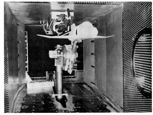
AIRPLANE and test vehicle shape models are positioned inside the Ling-Temco-Vought 4 ft. x 4 ft. high speed wind tunnel.
